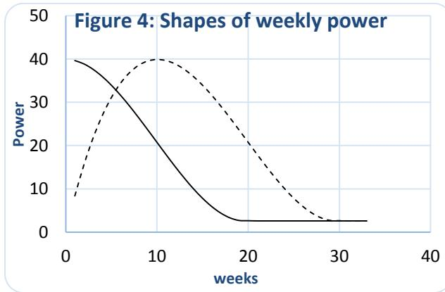
The shapes of the weekly power make clear that it is not constant over time. In this situation, we can define the work as the area underneath the curve, or in a mathematical formula:
